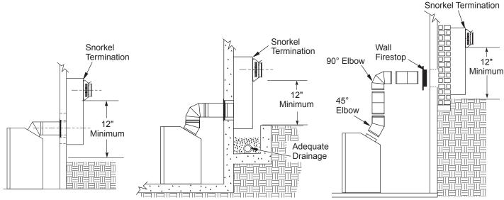
Figure 16 - Snorkel Termination Configurations for Below Ground Installation
